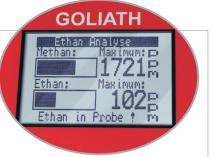
present in natural gas, whereas biogas (fermentation gas) does not contain any ethane at all. The device assesses the measurement result and also saves these data for future use.
